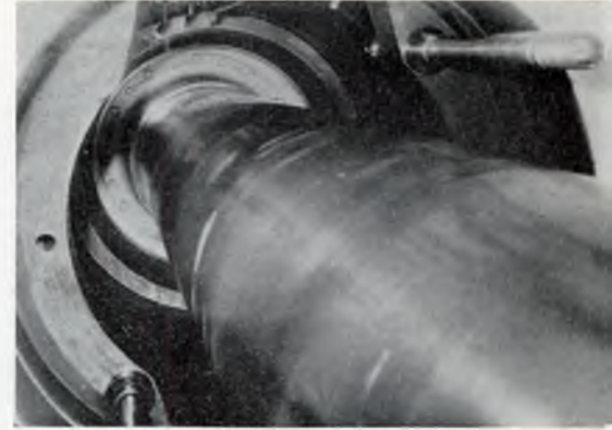
FIG. 10—The stern frame bearing recess—this shows the ample access space to the shaft surface and the outboard seal bush
