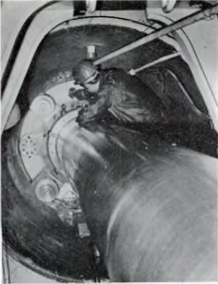
FIG. 8 (Left)—Commencement of the withdrawal operation FIG. 9 (Right)—Withdrawal of the bearing: the inboard seal has been removed along the shaft. The bearing has been jacked clear of its seating and is now being winched along the shaft.
