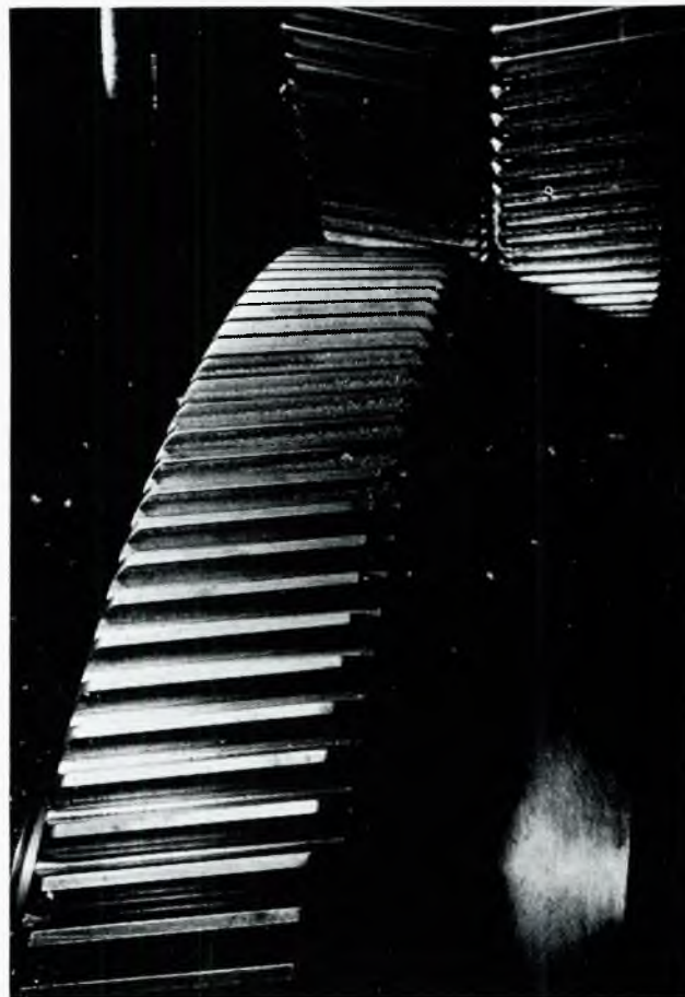
FIG. 17—Selective pitting on camshaft drive gears
