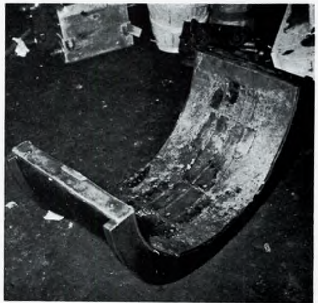
FIG. 31—Bearing shell damaged as a result of hammering
