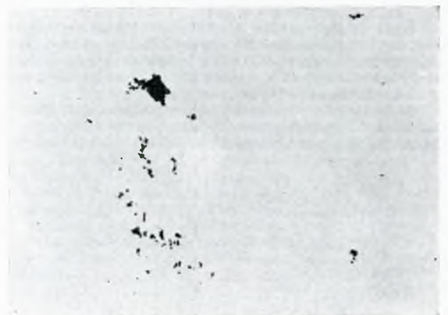
FIG. 10a—Mag × 100 non-etched—embedded impurities in fracture zone
