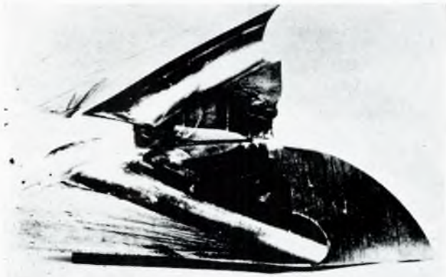
FIG. 14—Fracture at crankshaft oil hole
