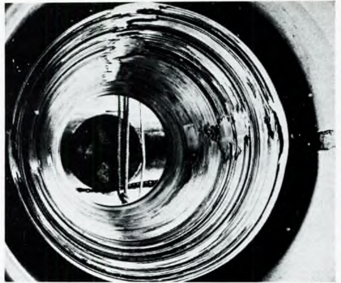
FIG. 23—White metal damage due to loss of contact at bush
