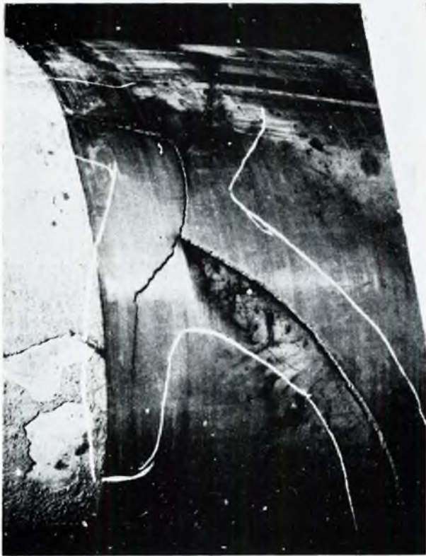
FIG. 22—Fractures of propeller shaft liners
