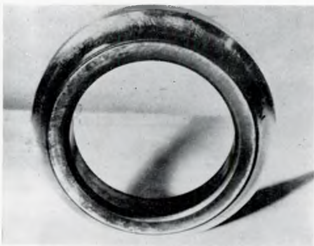
a) Damaged area on track of internal face
