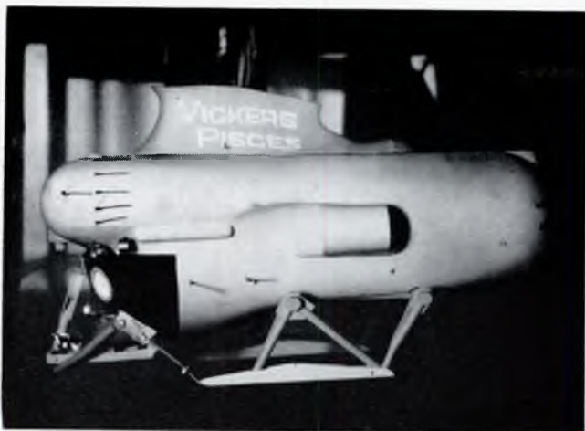
FIG. 6a—Model in cavitation tunnel showing present hull configuration
