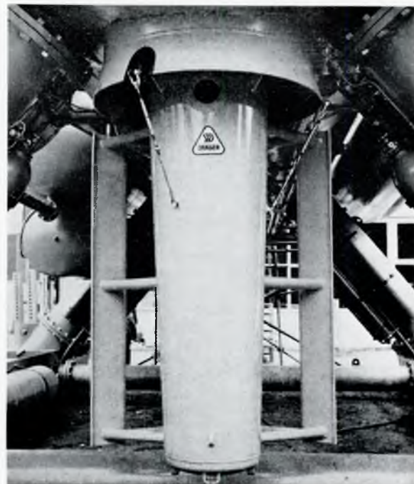
FIG. 6—One-man rescue chamber at UWL "Helgoland"
