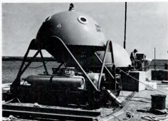
FIG. 7—Underwater igloo and depot prior to operation in the North Sea
