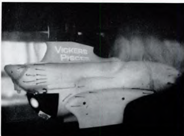
FIG. 6b—Model in cavitation tunnel showing various improvements to hull streamlining
