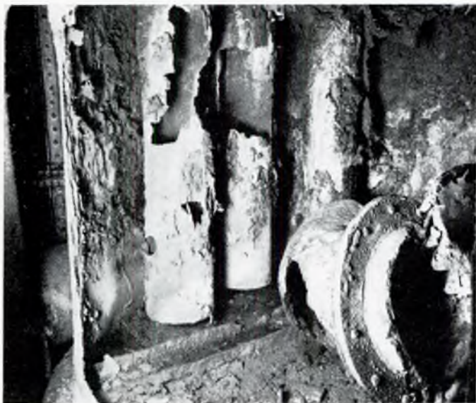
FIG. 25—Damage to gas scrubber on s.s. British Skill when inlet pipe failed
