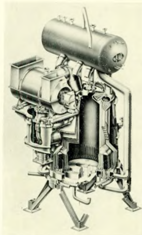
FIG. 2—Foster Wheeler supercharged steam generator
