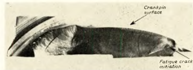
FIG. 4—Propagation of fatigue crack through angled oil hole in crankshaft
