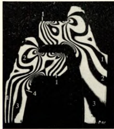
FIG. 8—Isochromatic photographs of two longitudinal sections disposed radially between two flange holes ( d=4.1 and 4.9 \text{ mm} respectively)
