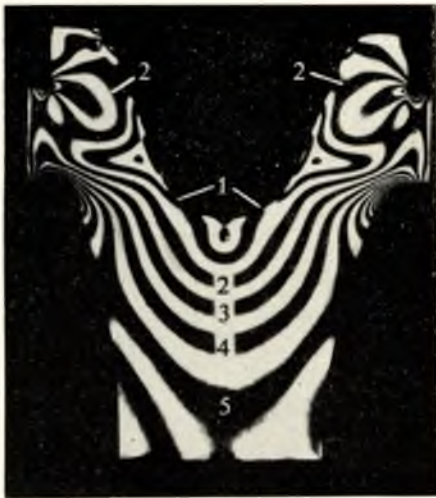
FIG. 7—Isochromatic photographic of the longitudinal section disposed at 90^\circ to the plane of symmetry ( d=6.8 \text{ mm} )
