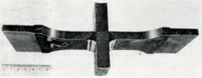
FIG. 28—Welding sample for fatigue tests
