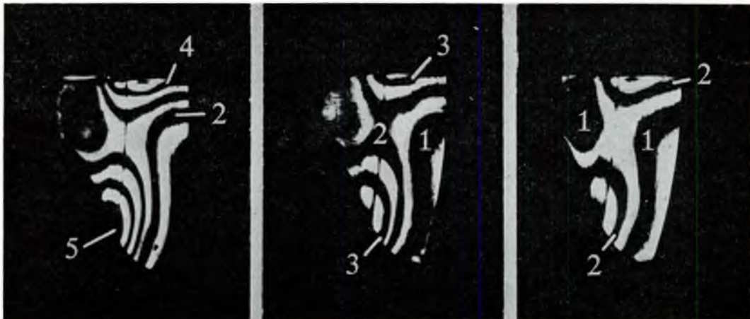
FIG. 3—Isochromatic photographs of the shell section "s" of Fig. 4, for three different section thicknesses
