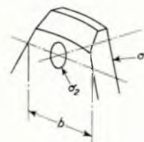
FIG. 30—Stresses at the edges of crank webs in torsional loading of crank throws
