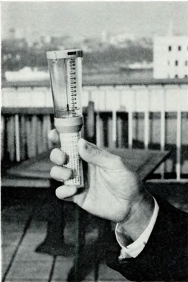
FIG. 8—A Ventimeter—a cheap, reliable maintenance-free instrument for measuring wind speed
