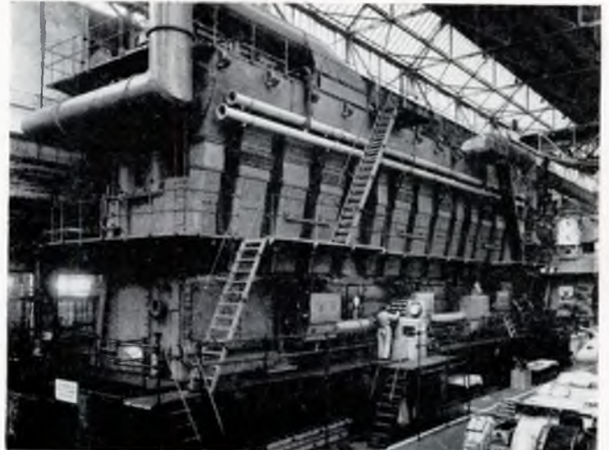
FIG. 4—The Fiat engine type 9012S on the test bed—In this case also the manoeuvre console is separate from the engine
