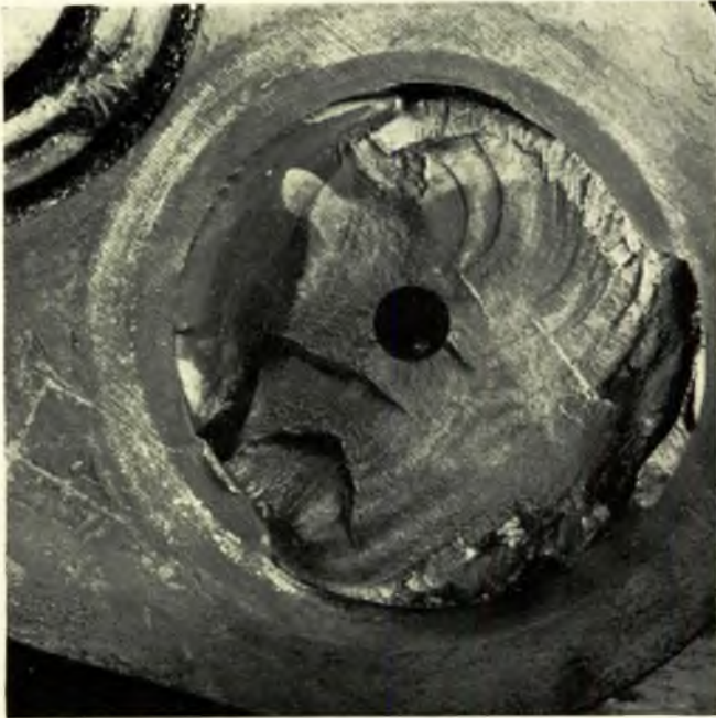
FIG. 17—Fatigue fracture section through No. 3 crankpin (forward) (Case V)
