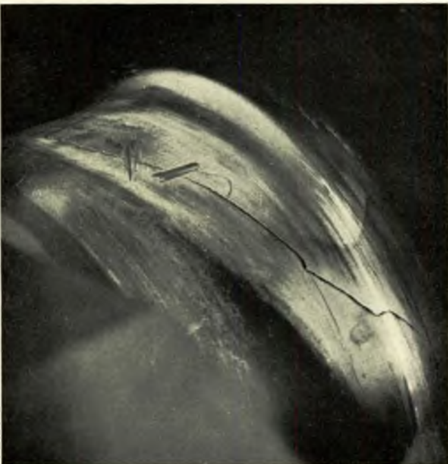
FIG. 18—Combined torsion/bending fatigue crack in No. 4 journal/forward web originating from welded repair (Case VI)
