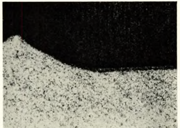
FIG. 8—Showing run-out of nitrided case in vicinity of radius (Case II)
