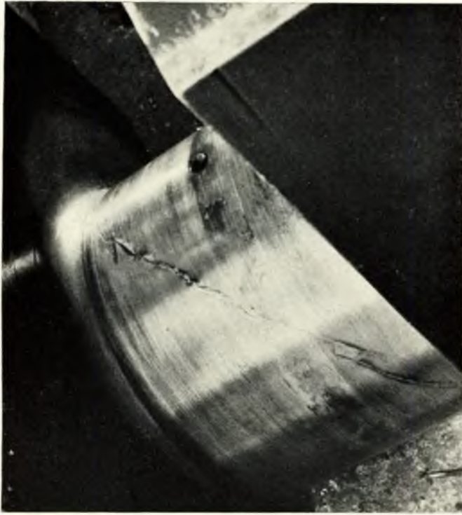
FIG. 6—Torsional fatigue fracture in No. 7 crankpin (Case I)
