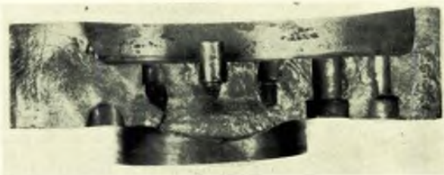
FIG. 11—Fracture section through No. 4 aft centre coupling/web (Case III)
