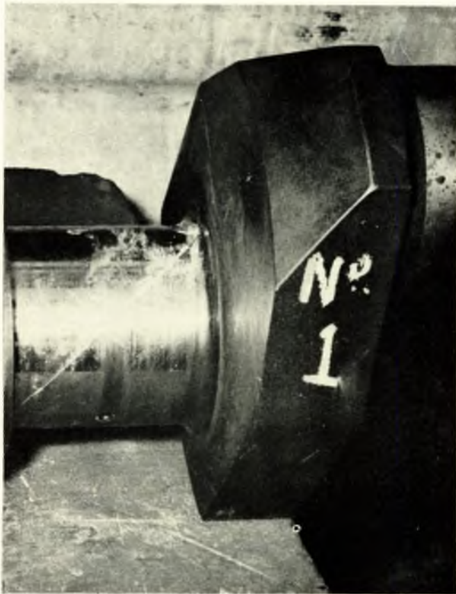
FIG. 24—Torsional fatigue crack clear of oil hole in No. 6 journal of five-throw auxiliary crankshaft (Case IX)
