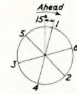
Crank positions for maximum B.M. at journal No. 2
