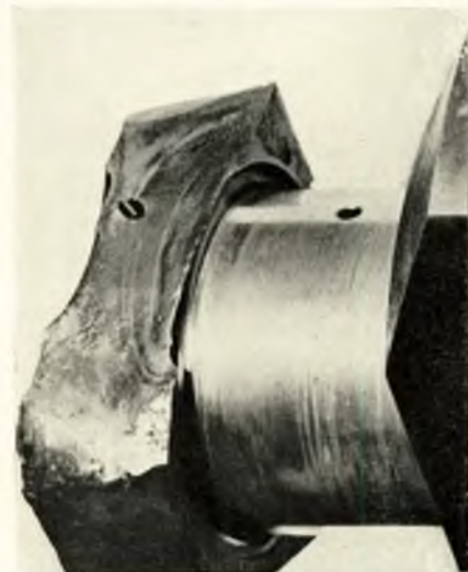
FIG. 21—Bending fatigue in auxiliary engine crankweb (Case VIII)
