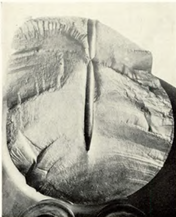
FIG. 13—Fracture section through No. 5 crankpin (Case IV)
