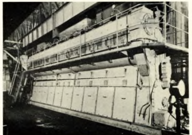
FIG. 22—G 10V 52/74 Diesel-gas engine
