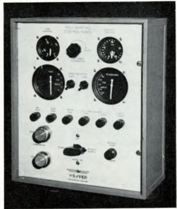
FIG. 6—Typical control panel for roll damping fin installation allowing complete remote control of equipment
