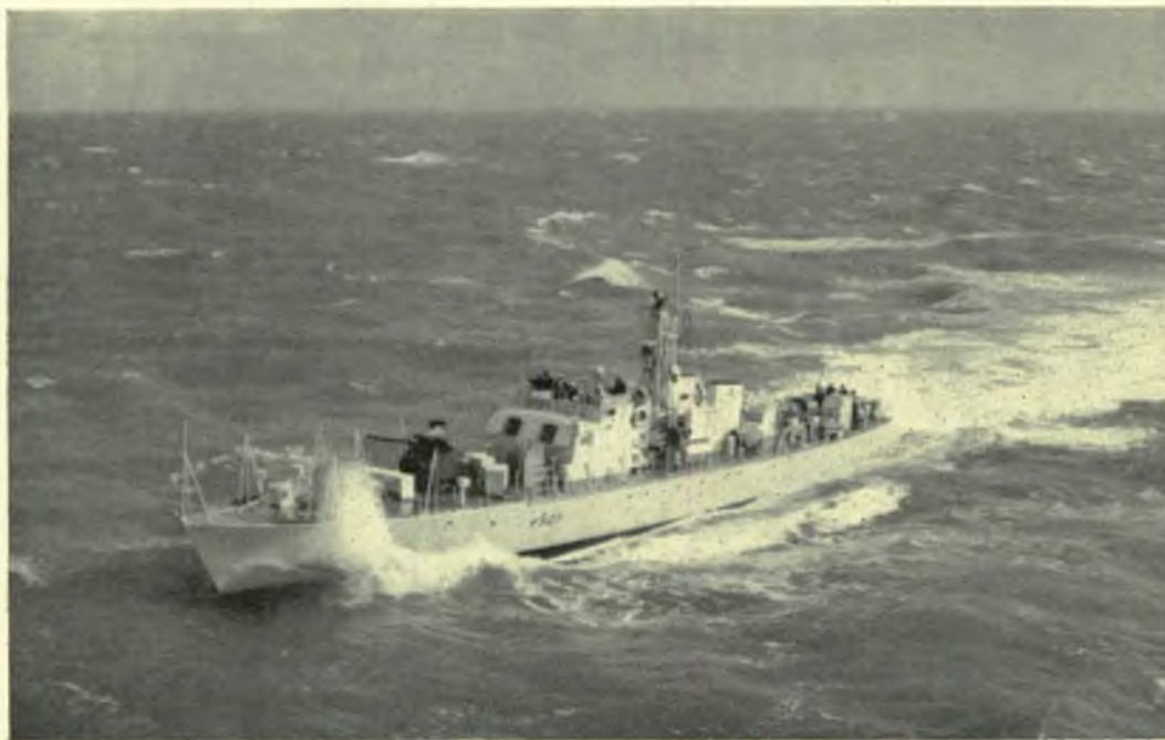
FIG. 10—S.A.S. Oosterland undergoing trials of her Vosper roll damping fins. This little ship has since made voyages to the Antarctic and Tristan du Cunha which would not have been considered feasible until the roll damping fins were fitted
