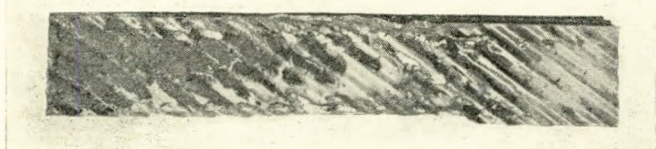
Second and subsequent vitreous enamelled elements undamaged (vitreous enamel damaged where fused to adjacent elements).
