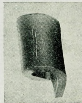
FIG. 3.—Intergranular corrosion cracks in wrongly treated austenitic steel containing 0.35% Carbon, 11.5% Chromium, 35.5% Nickel, after exposure to steam at 400° C. for 168 hours. The cracks became visible on bending the strip.
