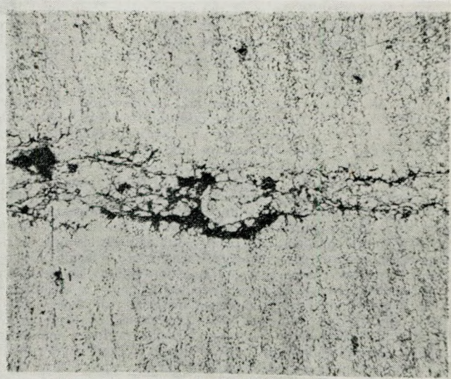
FIG. 1.—Intergranular corrosion cracks in wrongly treated "18-8" austenitic steel shrouding strip. This steel was not of the disintegration-proof type, and should not have been used for blading.
