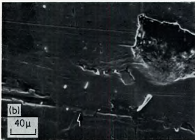
Higher magnification view of (a) showing surface flow across machining mark
