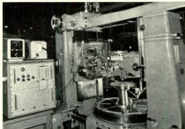
FIG. 3—Gear-hobbing machine fitted with grating measuring systems
