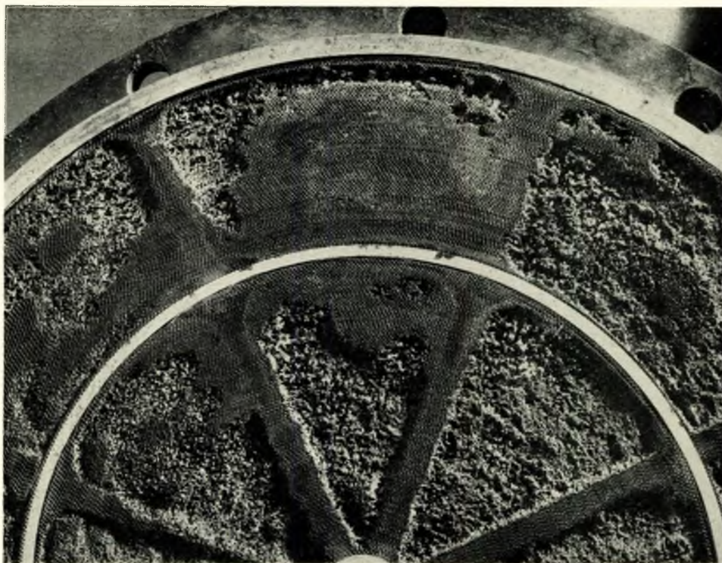
FIG. 4—Flame trap after Experiment 109 showing damaged areas
