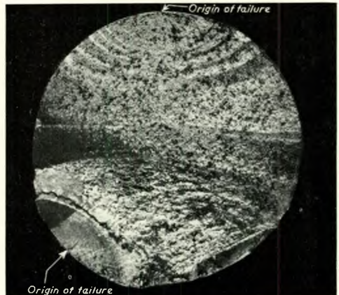
FIG. 5—Fatigue failure, starting turbine shaft
