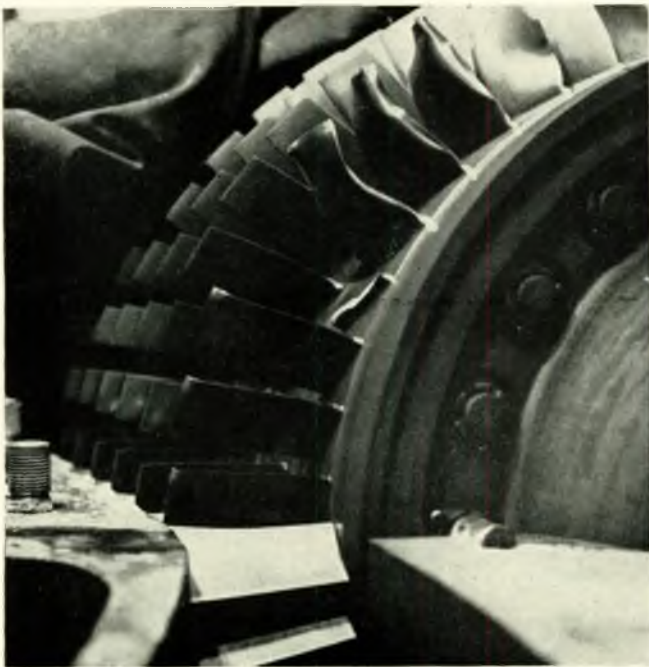
FIG. 17—Failure of L.P. compressor blades rotor
