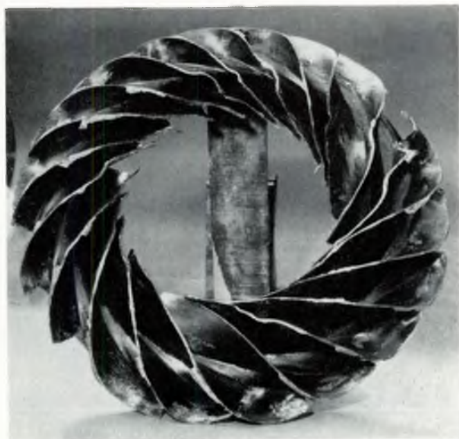
FIG. 6—Failure of hydraulic converter
