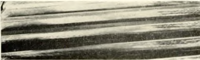
FIG. 8—Main wheel of 1st unit on completion of trials with E.P. oil
