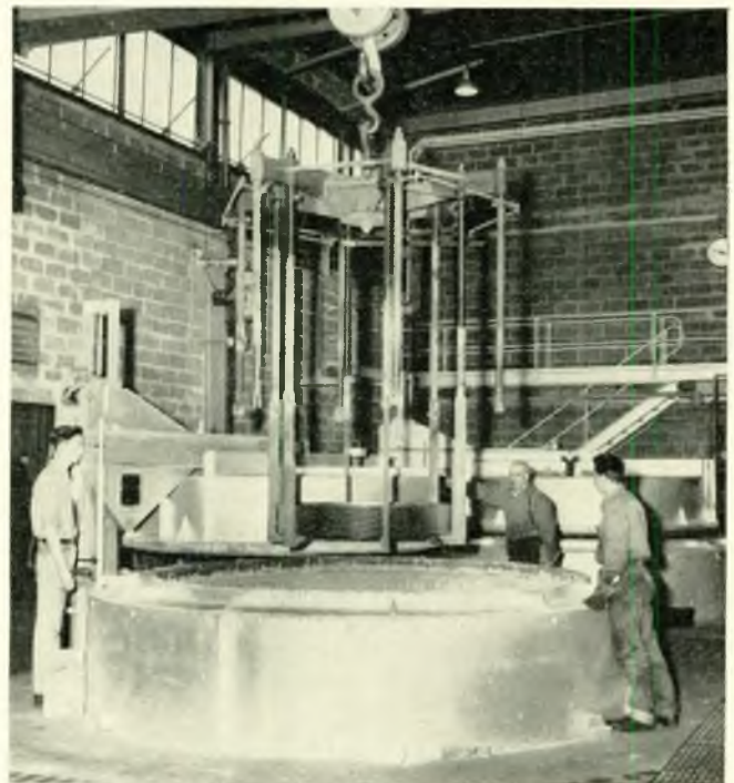
FIG. 11—Primary reduction gear rim entering carburizing furnace
