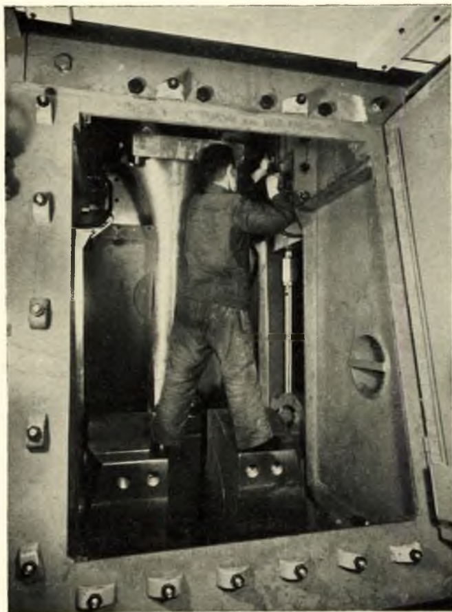
FIG. 29—Inspection work inside crankcase
