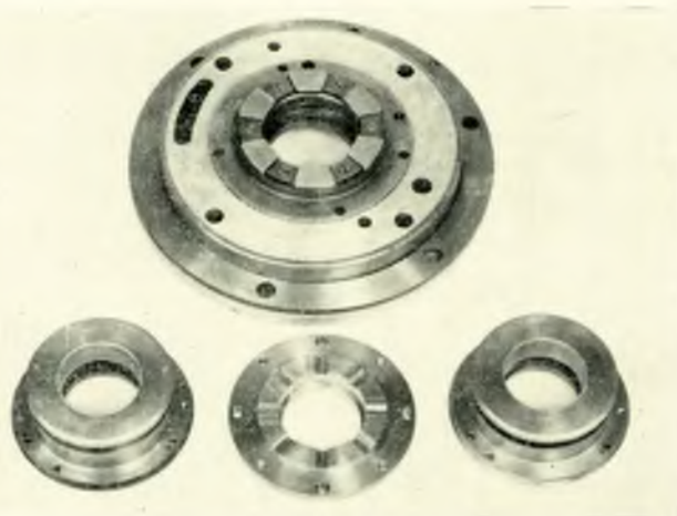
FIG. 51—50 series turbocharger journal and thrust bearing assemblies after 1,200 hr. test
