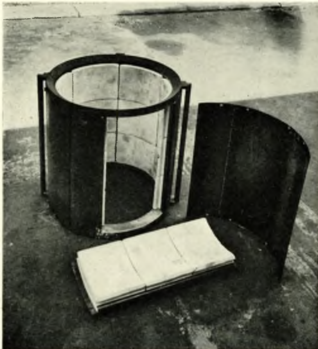
FIG. 7—Ceramic lined flame tube
