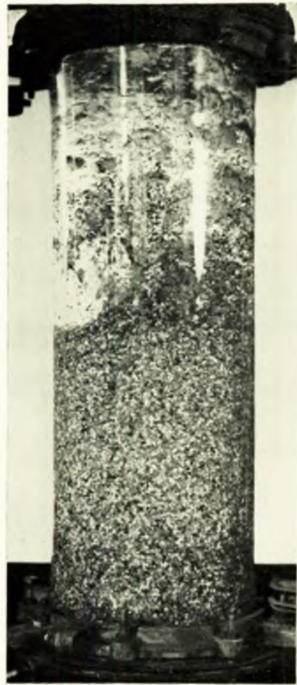
FIG. 24—Conditions in the filter bed during the cleaning phase
