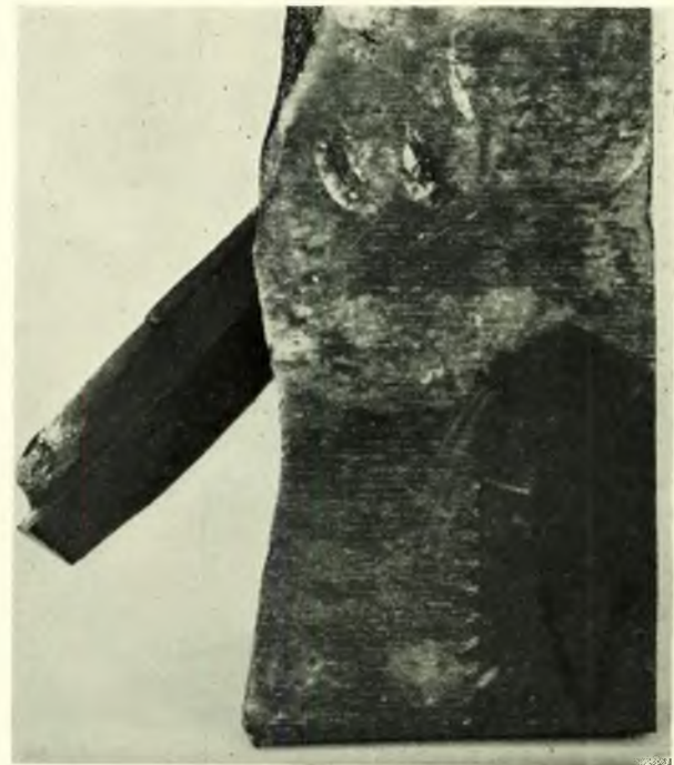
FIG. 8—Rim marking from un-filled dowel hole
