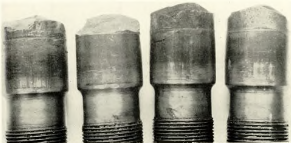
FIG. 24—Fretting corrosion failure of coupling bolts
