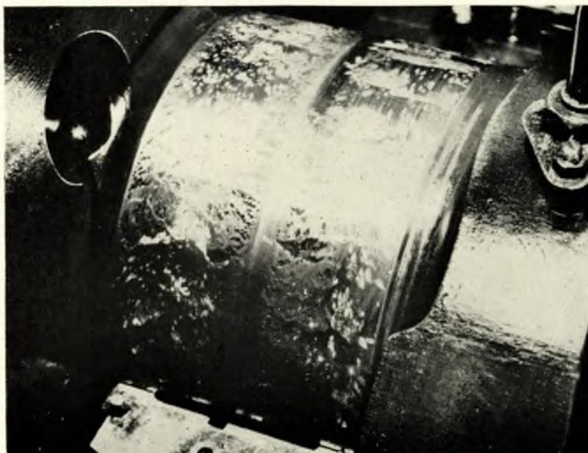
FIG. 31(a)—Damage to journal and crank pin due to contaminated lubricating oil
