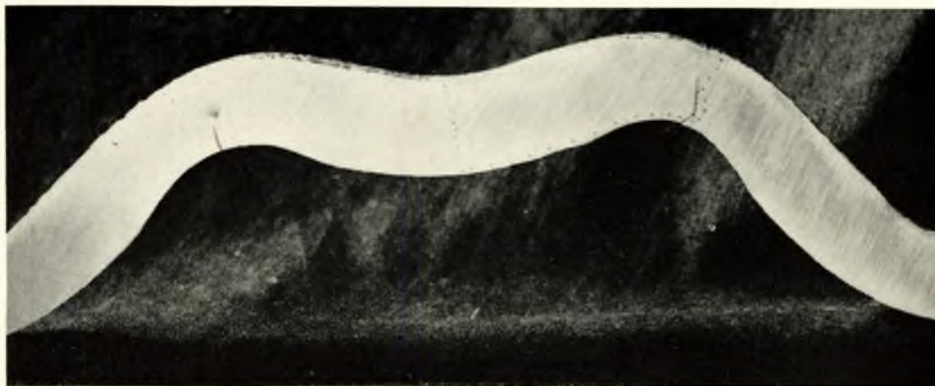
FIG. 30—Cracks in the furnace corrugations
