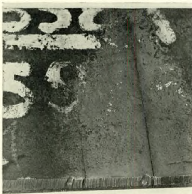
FIG. 18—Cracking of flame cut plate
