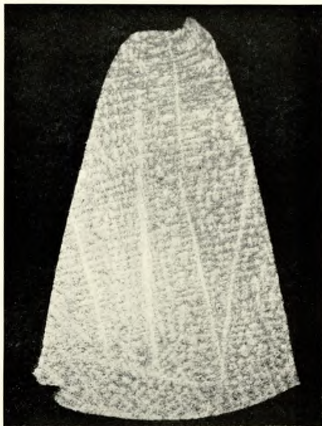
FIG. 10—Gear tooth showing dendritic structure
