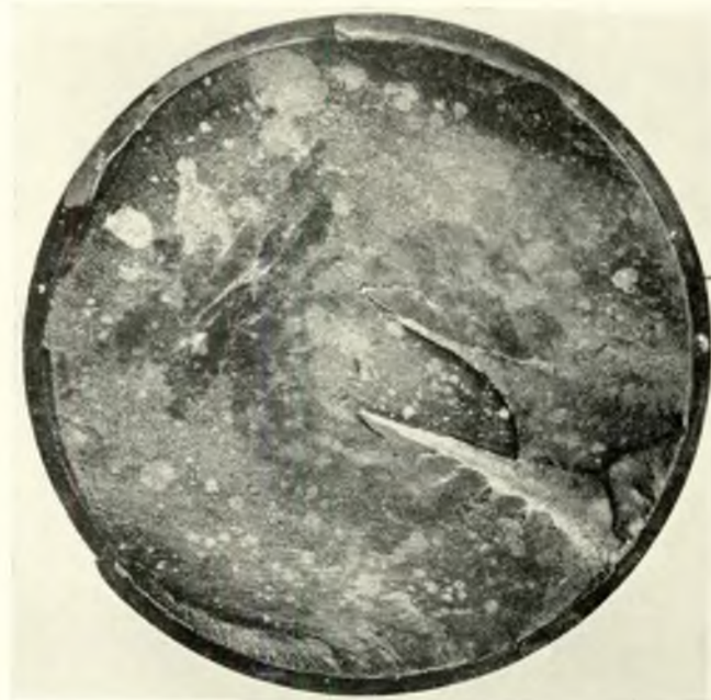
FIG. 26—Corrosion fatigue failure of tie rod
