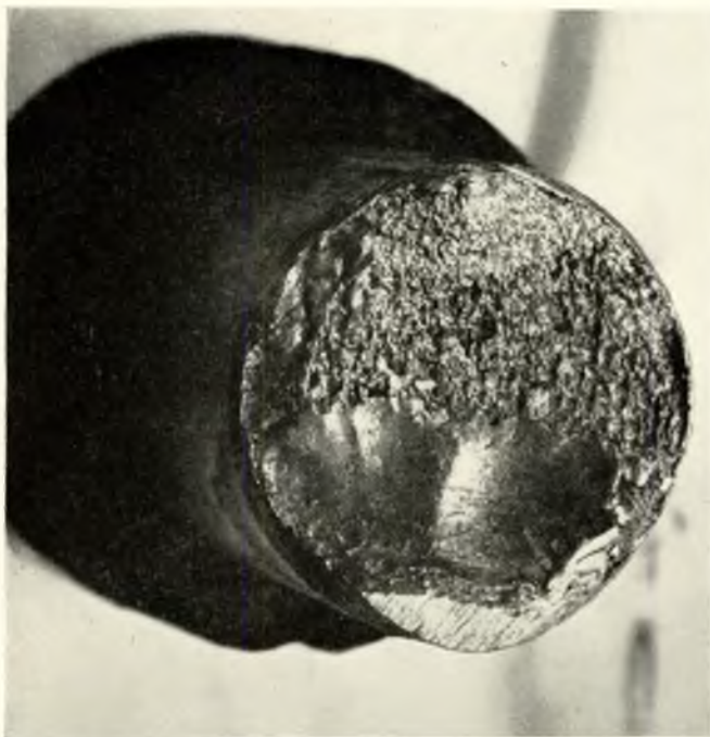
FIG. 23—Coupling bolt failure
