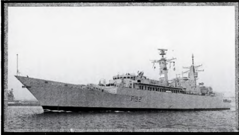
Fig. 1(c). HMS Boxer , a Type 22 frigate using rivetted joints
