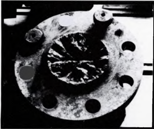
Fig. 2. Multi-origin intermediate shaft fracture
