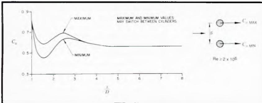
Fig 11: The effect of lateral spacing on the drag coefficient of cylinders in a side by side arrangement
