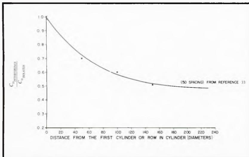
Fig 16: The effect of shielding on successive in-line cylinders
