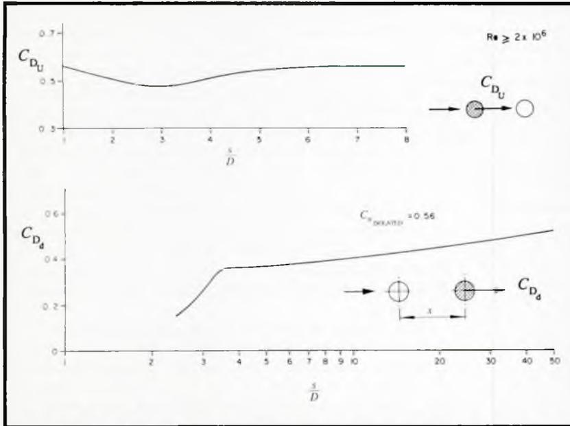
Fig 12: The effect of longitudinal spacing on the drag coefficient of cylinders in tandem
