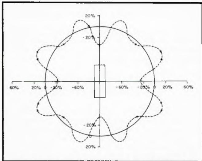
Fig 18: Comparison of the average drag coefficient on a group of conductors with that on an equivalent isolated cylinder
