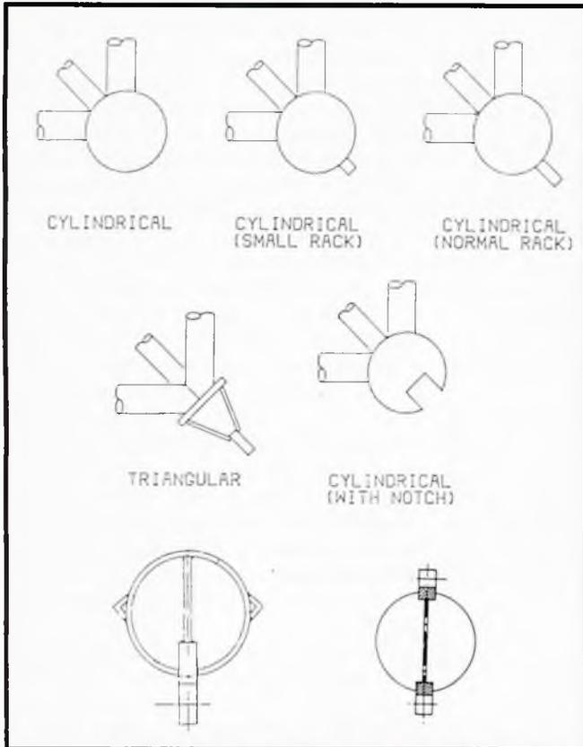
Fig 10: Range of possible corner posts on jack-up legs
