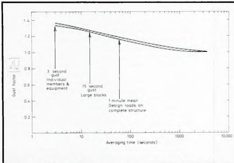
Fig 3: Gust factors for winds over the sea – relative to the 1 h mean wind at 10 m above sea level
