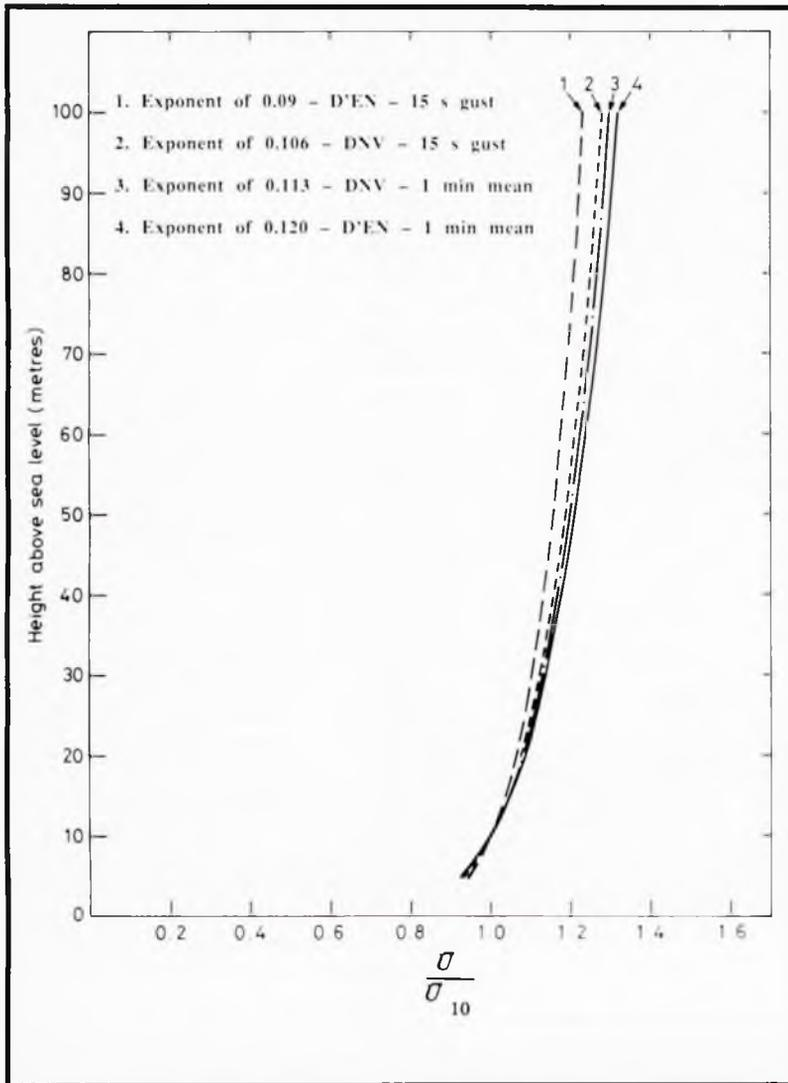
Fig 5: Profile of velocity over the sea for various power laws
