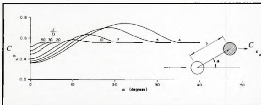
Fig 14: The effect of flow interference on the drag coefficient of downstream cylinders in a staggered arrangement
