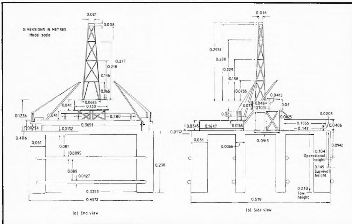
Fig 19: Line sketch of a SEDCO 700 used during model tests (from ref 37)
