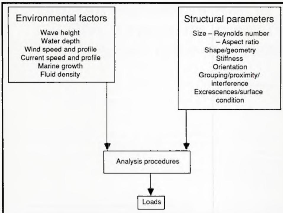
Fig 1: Routes to estimating fluid loading
