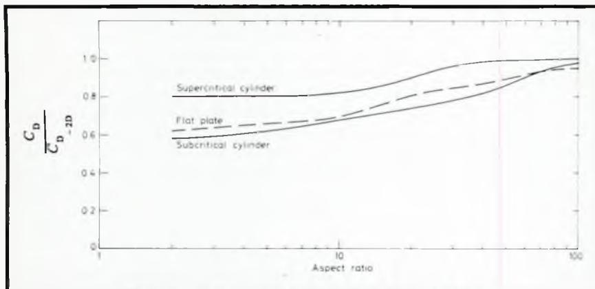
Fig 7: Effect of aspect ratio on drag coefficient
