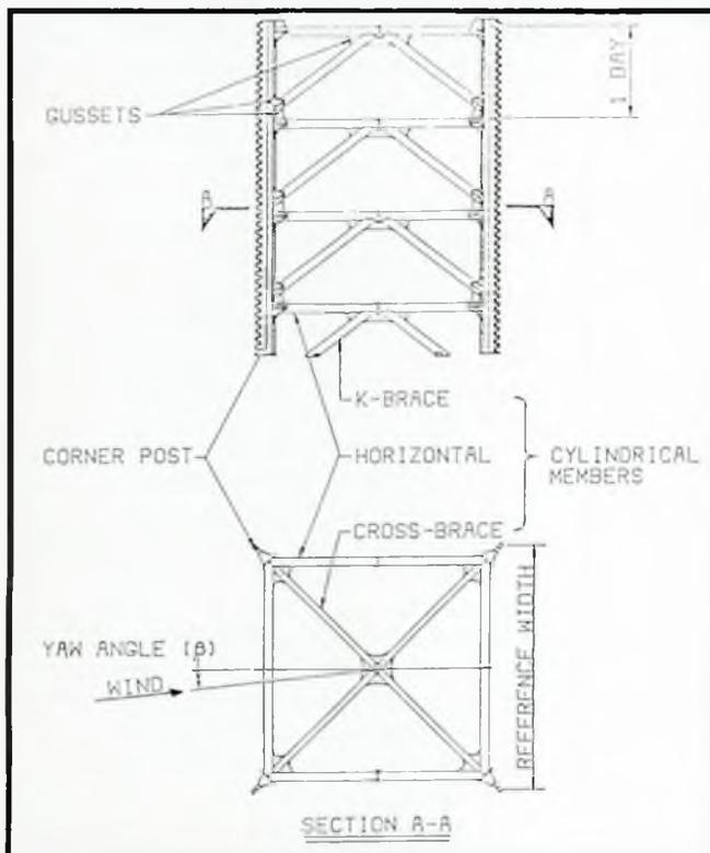
Fig 9: Typical leg section of a jack-up unit (from ref 27)
