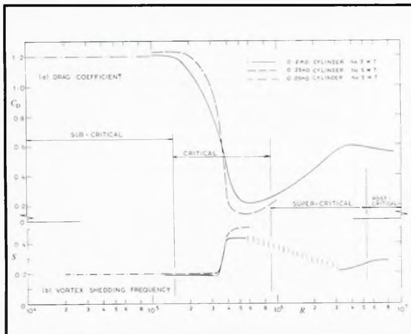
Fig 6: Variation of drag coefficient and vortex shedding frequency with Reynolds number (from ref 16)
