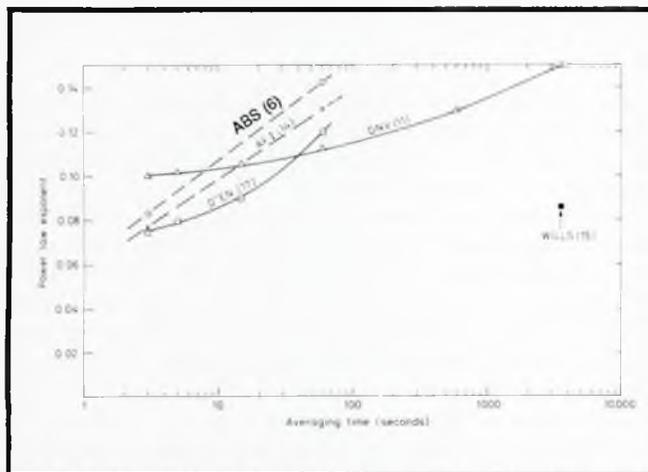
Fig 4: Recommended values for power law exponent for wind shear over the sea
