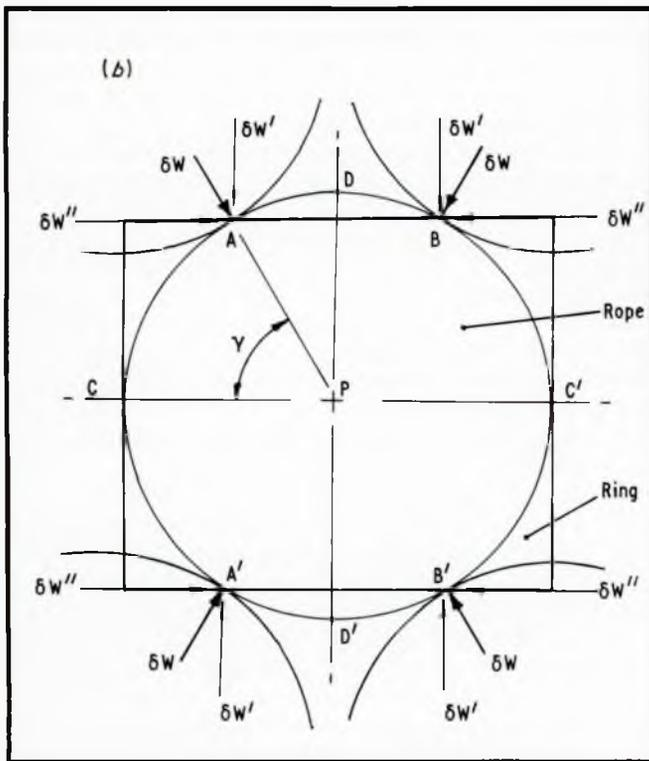
Fig 1: (a) The rope and (b) its ring model for all layers except the first
