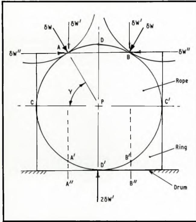
Fig 2: The rope and its ring model for the first layer
