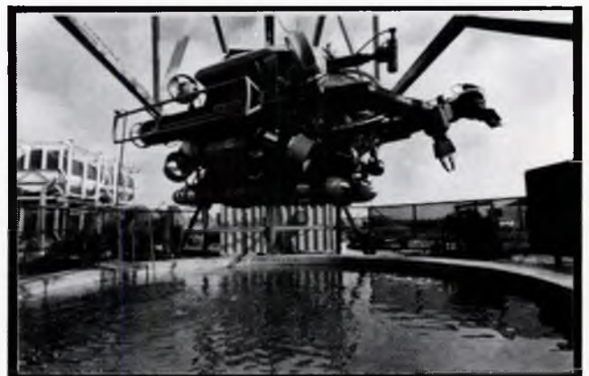
Fig 3: Duplus prototype with vectored thrusters
