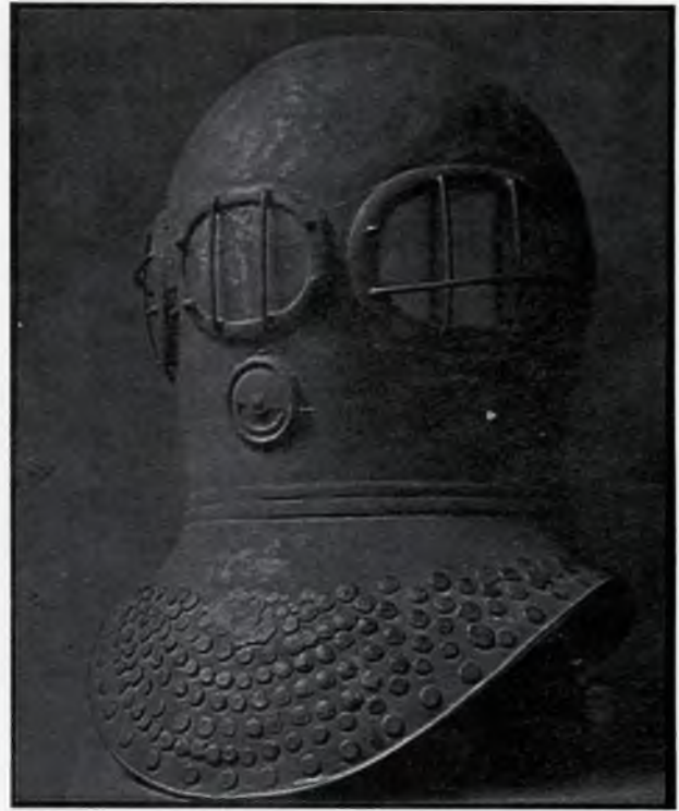
Fig 7: Siebe's first 'open' diving helmet (1819)
