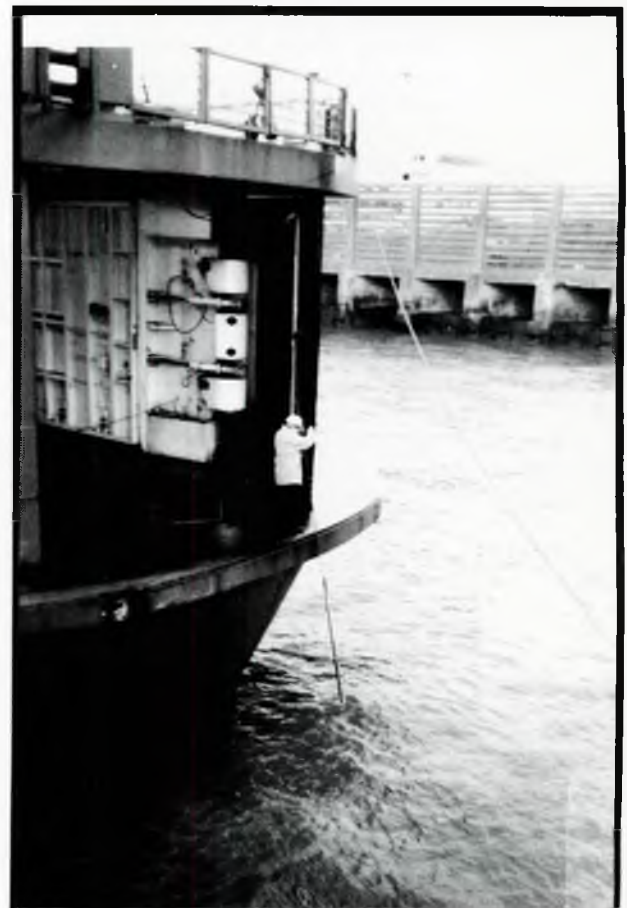
Plate 3: Using dipstick to read draught Forward draught marks can be seen at an acute angle.
