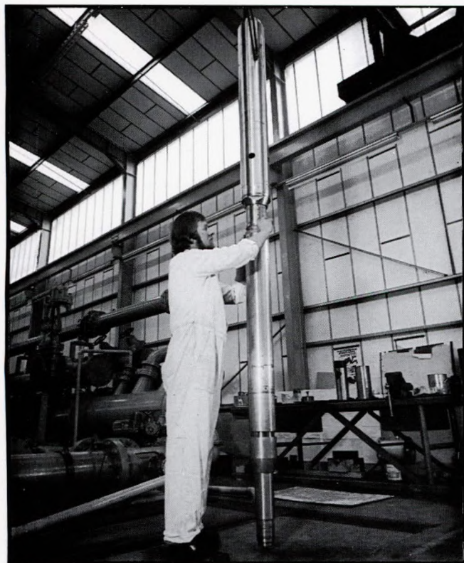
FIG. 11: 16,000 barrels/day, 315 h.p. downhole pumpset
