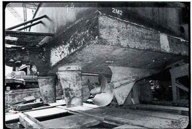
Fig. 2 (b). General view of underwater appendages
