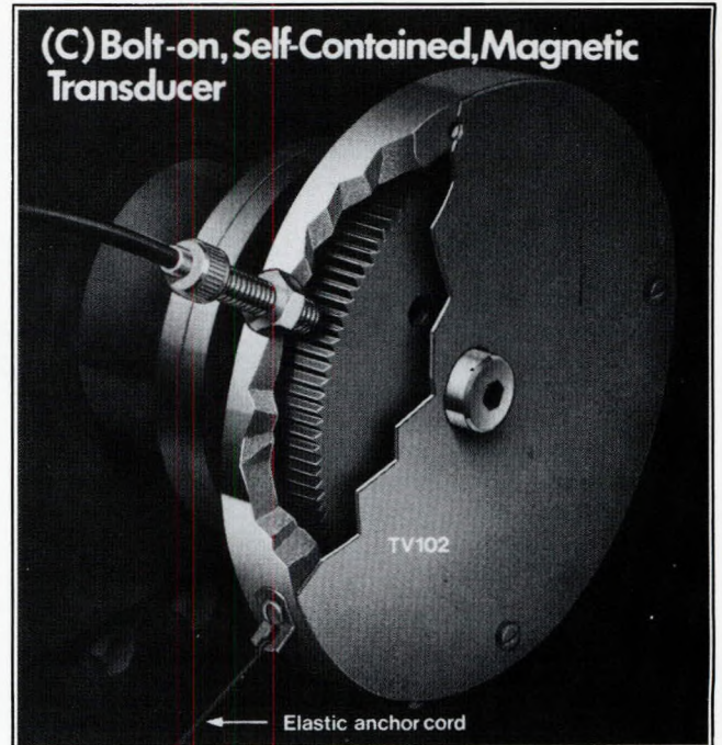
FIG. 5: Arrangement of Econocruise system for vibration analysis
