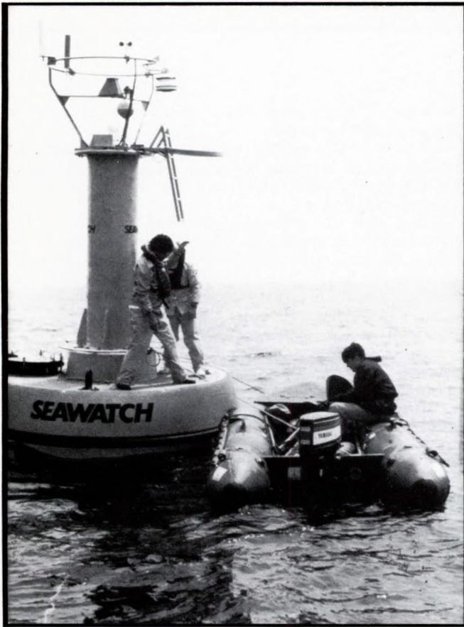
FIG. 10: The new low-cost, lightweight Seawatch databuoy which transmits data by either VHF or satellite
