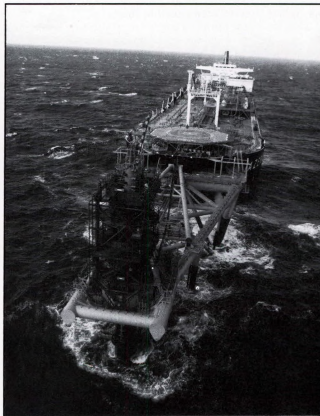
FIG. 3(b): Murex after conversion to Tazerka FPSU
