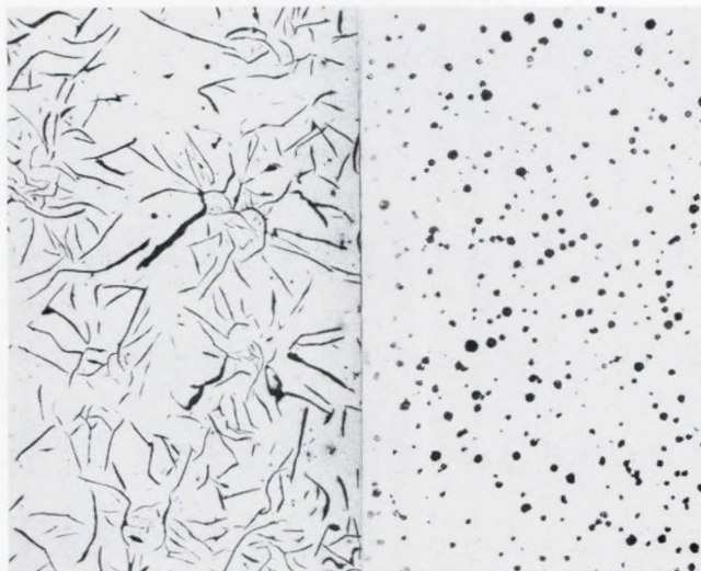
FIG. 28 Flake cast iron (left) and nodular cast iron (right)
