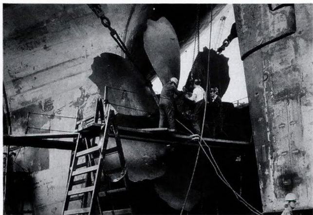
FIG. D9 Damaged six-bladed propeller
