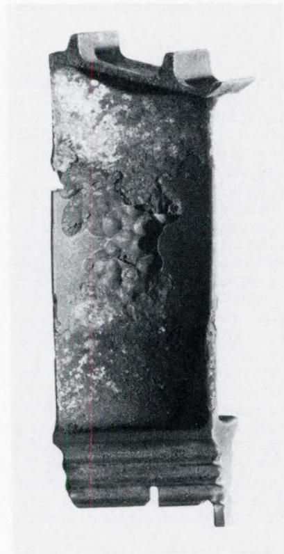
FIG. 11: Corroded gas turbine rotor blade
