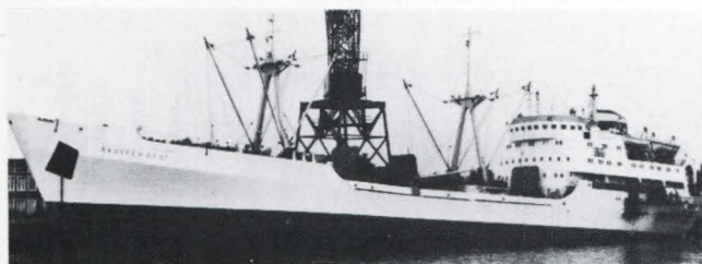
FIG. 12: One of five fishery ships with original main engines replaced by 4 × 6ASL25H operating on HFO
