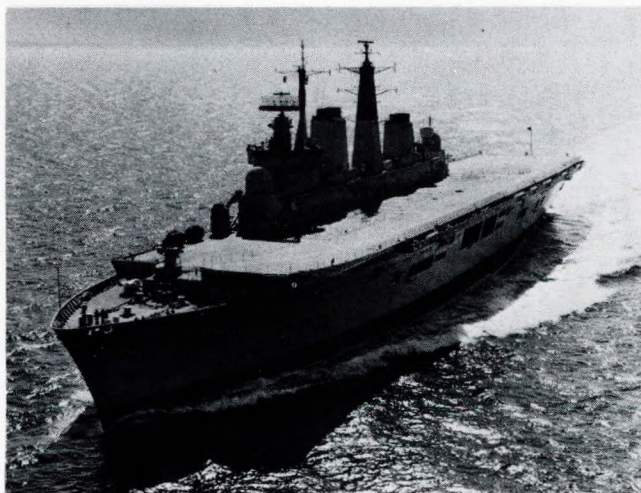
FIG. 16 HMS Invincible : powered by four Olympus gas turbines
