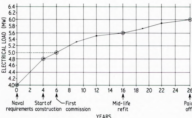
FIG. 1 Growth of electrical connected load from original concept until end of ship's life
