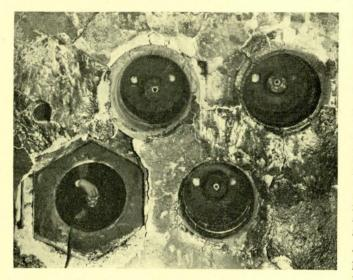
FIG. 31.—"Carbofrax" segments—s.s. Peleus—after two years' service
