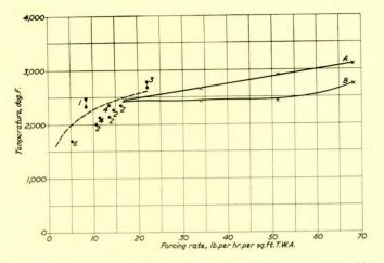
FIG. 30—Comparison of naval boilers with merchant ship boilers
