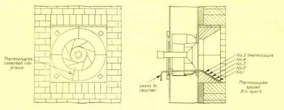
FIG. 12—Arrangement of thermocouples in quarl block, boiler 9
