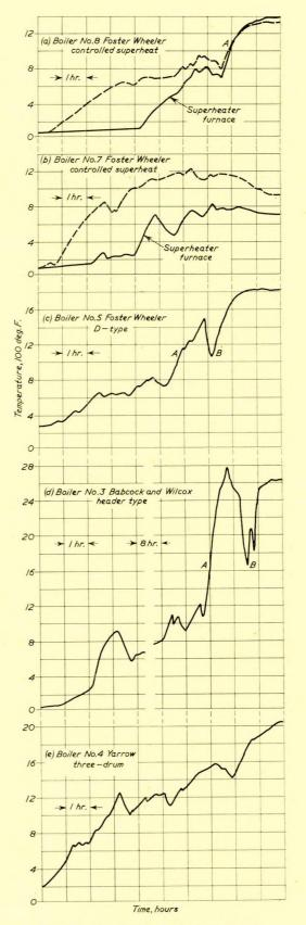
FIG. 11—Typical records of back wall temperatures during steam raising and manœuvring
