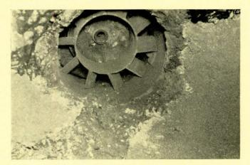
FIG. 23—Burner quarl showing repeated patching leading to loss of shape and misalignment (three years' service)
