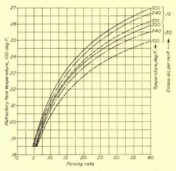
FIG. 5—Effect of excess air and air temperature on refractory temperature. Exposed walls—short flame burning
