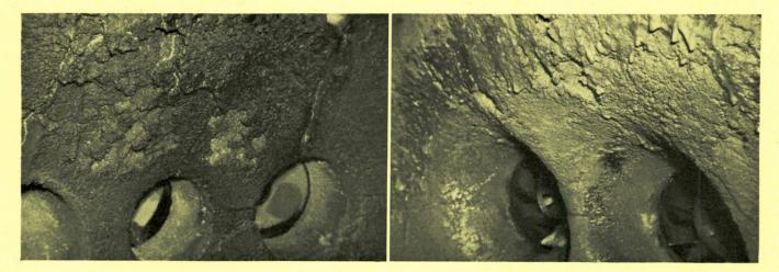
FIG. 26 FIG. 27 Spalling damage to upper surfaces of dish shaped burner sections
