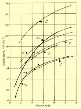
FIG. 9-Effect of water wall tubes on refractory hot face temperature-long flame burners. (Curves drawn for air at 240 deg. F., 2-in. outside diameter tubes)
