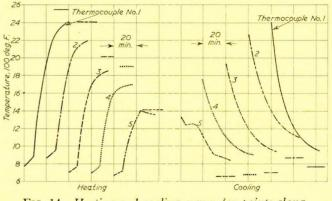
FIG. 14—Heating and cooling curves for points along quarl block, boiler 9
