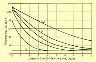
FIG. 2—Typical temperature gradients through 9-in. header brick
