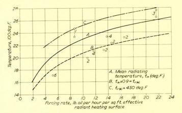
FIG. 3—Maximum refractory hot face equilibrium temperatures. Test results from boilers with exposed walls (air at 240 deg. F.) (Numbers adjacent to points indicate boiler number)
