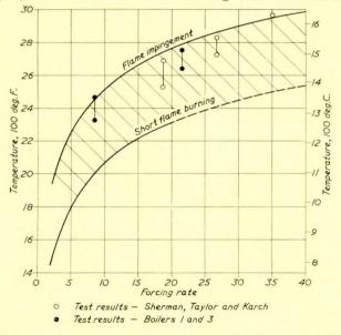
FIG. 4—Maximum refractory hot face equilibrium temperatures: exposed walls. Air temperature 240 deg. F., excess air 30 per cent
