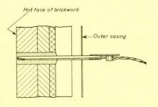
(b) IN WALL OF BOLTED BLOCK CONSTRUCTION
