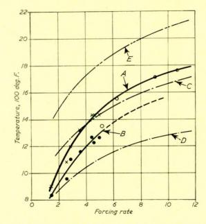
FIG. 10-Effect of water wall tubes on refractory hot face temperature-short flame burners. (Curves drawn for air at 240 deg. F., 2-in. outside diameter tubes)
