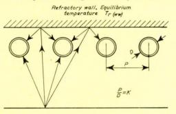
Radiating plane temperature T<sub>r(e)</sub> = temperature of exposed refractory wall
