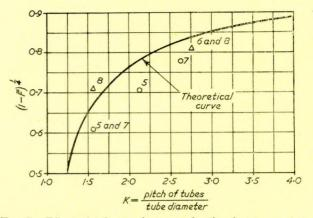
FIG. 7—Effect of tube spacing on reduction in temperature of refractory, compared with exposed wall
