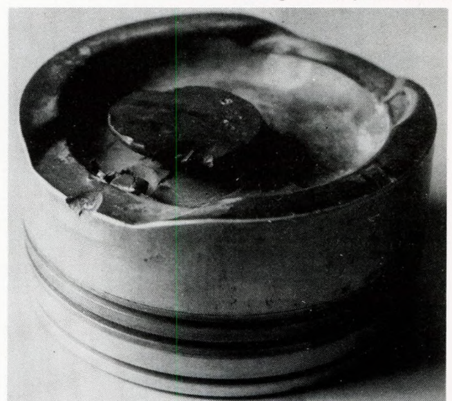
▼ FIG 4 Diesel generator piston failure
