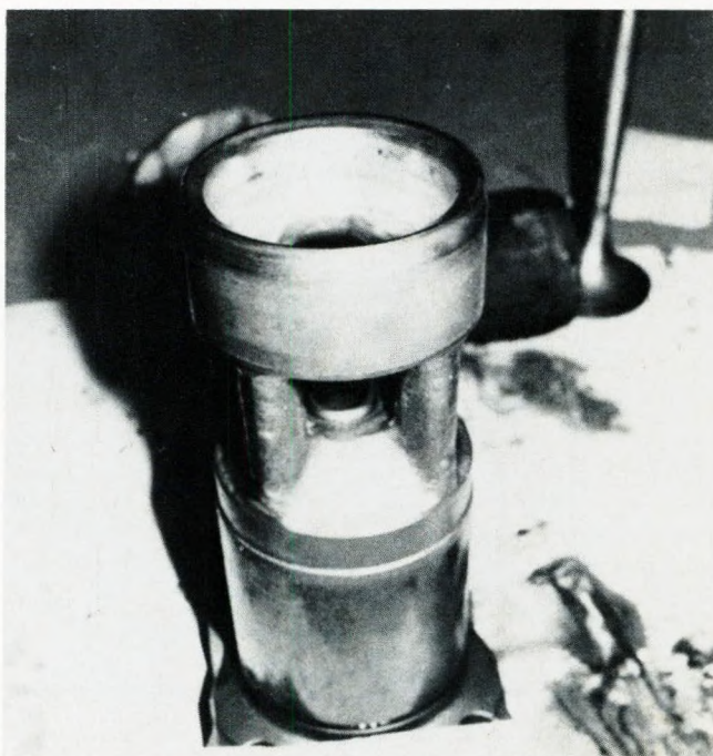
FIG 27 After blasting in cleaning cabinet
