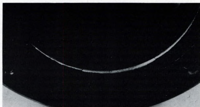
Fig. 10c Kootenay pinion for'd bearing end rubbing contact
