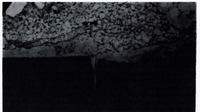
Fig. 13b Enlarged area showing penetration of molten thrust bronze into steel backing ring
