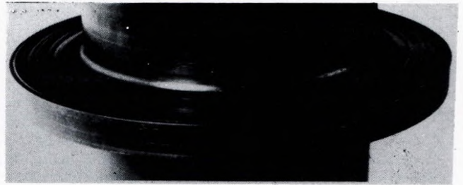
Fig. 12 Kootenay pinion thrust collar wear
