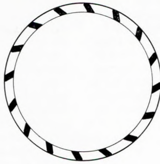
(b) Modified Scavenge Ports with no Swirl Vanes. This gave best results with two injectors.
