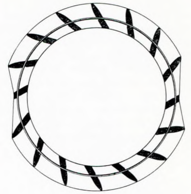
(c) Modified Scavenge Ports with Swirl Vanes.
