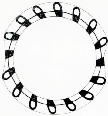
(a) From Seahorse Engine. Used initially with two injectors and finally with four injectors.
