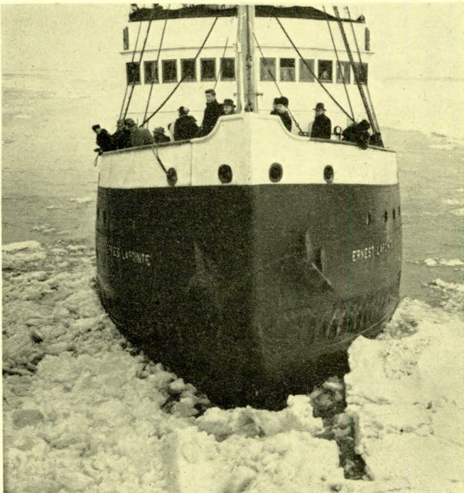
FIG. 12—Icebreaker Ernest Lapointe showing wall sided construction for buoy work
