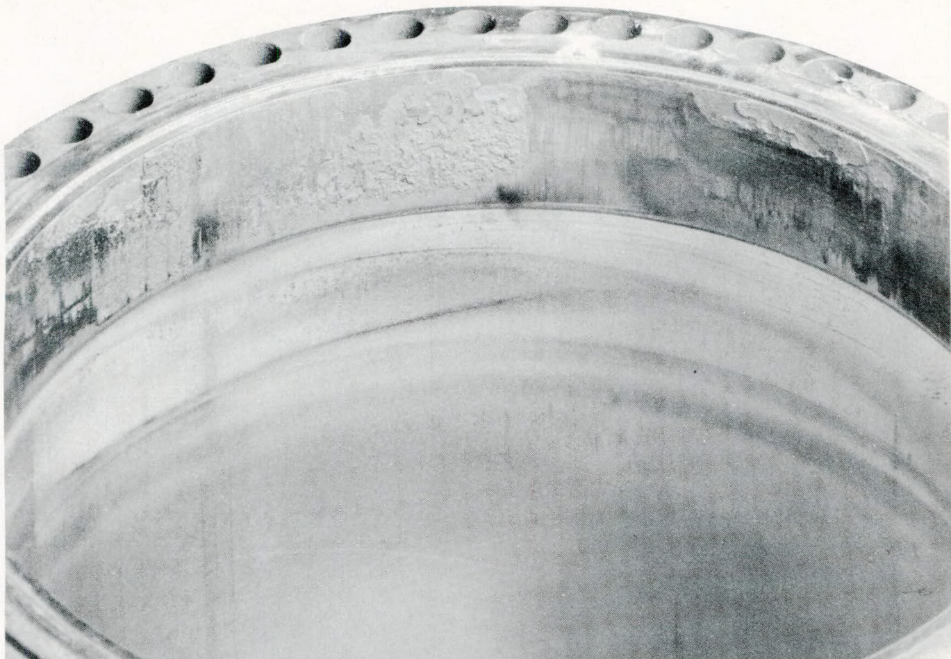
Fig.7—View of top of cylinder liner showing unusual staining in the vicinity of the top ring reversal position
