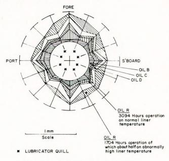
FIG. 12 — M.T. Esso Castellon — Liner wear configuration opposite third ring in TDC
