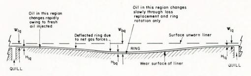
$H_{bq}$  and  $H_{lq}$  ~ Oil film thickness and variable with time
