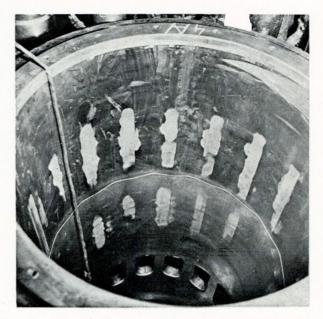
FIG. 17—Clover-leafing (corrosive) wear on chromium-plated cylinder liner
