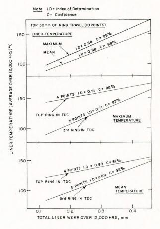
FIG. 10 — M.T. Esso Castellon — Relationship of liner temperature to wear
