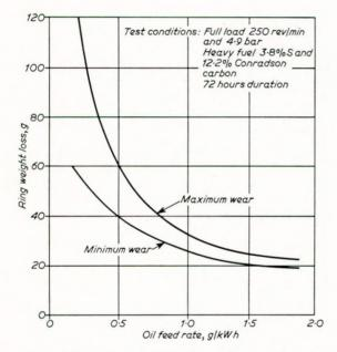
FIG. 16 — Influence of cylinder oil feed rate on piston ring wear (Sulzer T48 engine)
