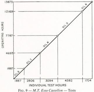
sequence in instrumented liner
