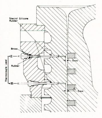
FIG. 8 — M.T. Esso Castellon — Details of thermocouples in upper half of liner
