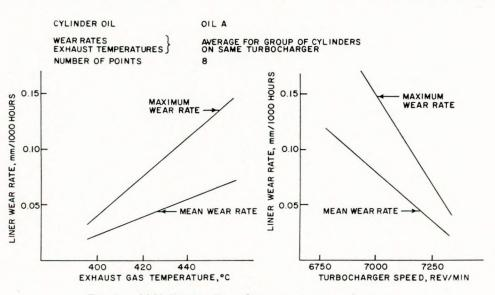
FIG. 2 — M.V. Strathardle — Liner wear rate vs exhaust gas temperature and turbocharger speed
