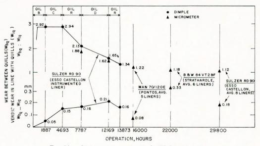
FIG. 14 — Liner wear at top ring in the TDC position areas between quills compared to in line with quills
