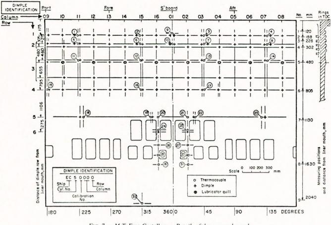
FIG. 7 — M.T. Esso Castellon — Details of thermocouples and dimples lay-out
