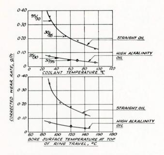
FIG.18-Effect of jacket temperature and lubricant on wear
