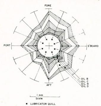
FIG. 11 — M.T. Esso Castellon — Liner wear configuration opposite top ring in TDC
