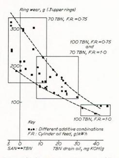
FIG. 15—Relationship between piston ring wear and Total Base Number (TBN) or Strong Acid Number (SAN) of cylinder oil drainings (Sulzer 2RF68 engine)
